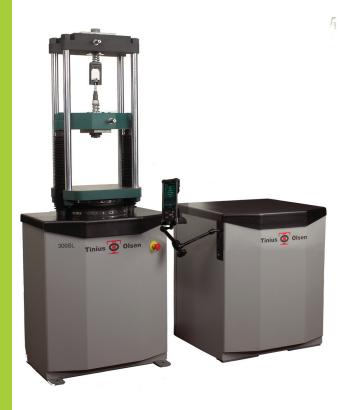
The Model 300SL is designed for tension, compression, flexure and shear strength testing on materials and assemblies. The robust design incorporates quality materials and components to ensure that our reputation for superior system performance, ease of use and longevity is maintained.
