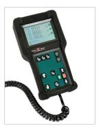
Familiar handheld interface that is tethered to the machine. With its larger, tactile, sealed keypad, this interface is ideal for operators who use gloves to load and unload specimens and prefer a push button keypad. It requires virtual machine control software running on a connected PC to operate the basic machine functions and report basic numerical test data.
