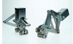
use two knurled rollers. The grip is particularly efficient for testing flexible dumbbell specimens. The centreline of the specimen remains constant in relation to the test machine, irrespective of the specimen thickness.
