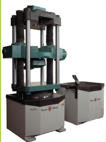
The Model 1500SL is designed for tension, compression, flexure and shear strength testing on materials and assemblies. The robust design incorporates quality materials and components to ensure that our reputation for superior system performance, ease of use and longevity is maintained.
